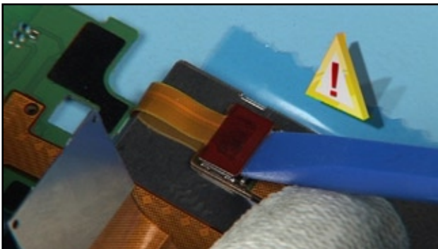
49. Gently open the flex connector. Avoid putting pressure to the components.
